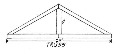
a) Calculate the length of the remaining sides of the truss.
